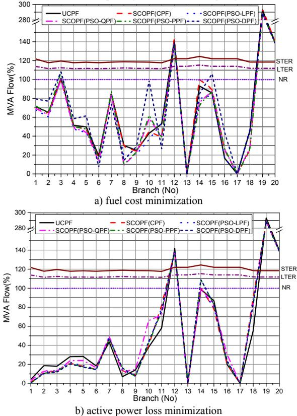
Fig. 6. Line MVA flows for unconstrained power flow solution and five PSO solutions with different penalty functions (contingency L6-13 and L9-14)
