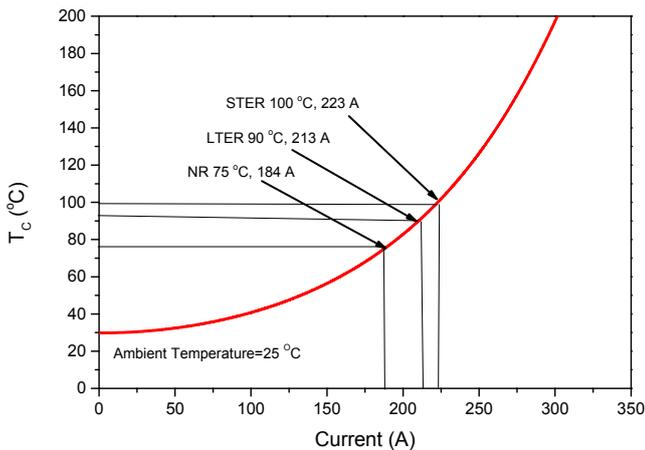
Fig. 1. Equilibrium conductor temperature,  $T_c$ , as a function of its current, [12]
