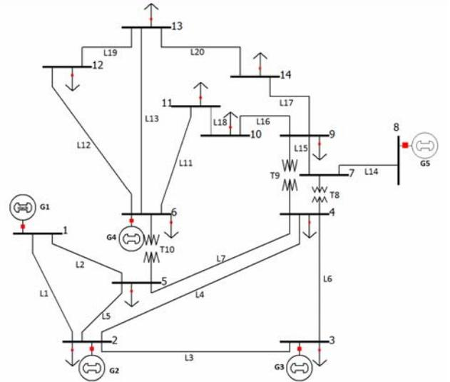
Fig. 4. IEEE 14-bus test network [16]
