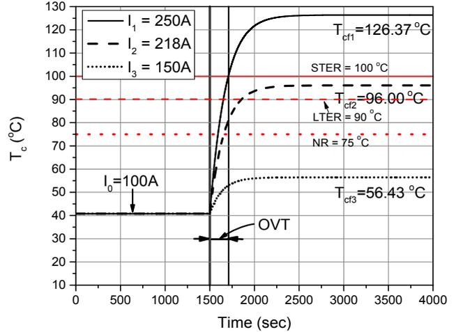
Fig.2. Illustration of the calculation of allowed overloading time (OVT)
