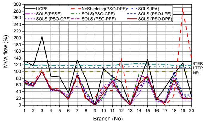
Fig. 7. Line MVA flows with and without load shedding for fuel cost minimization (contingency L6-13 and L9-14)
