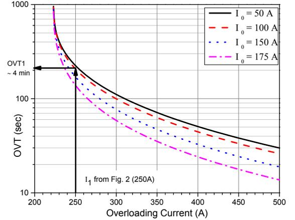
Fig. 3. Calculation of OVT: Different curves correspond to different pre-contingency currents, while post-contingency currents are on X-axis
