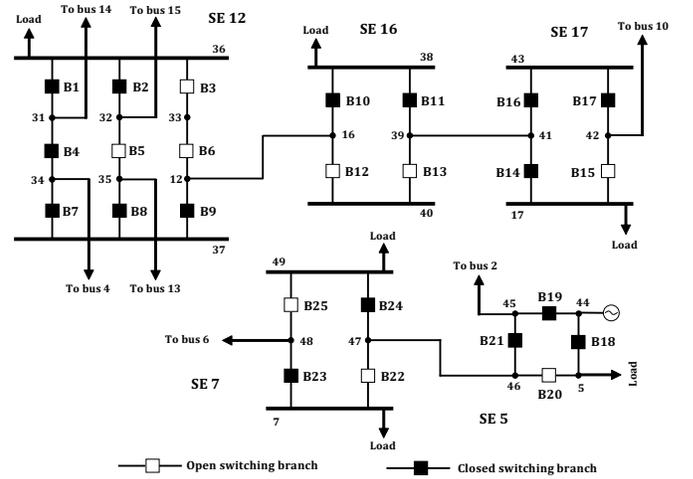
Fig. 3. Details of substations 5, 7, 12, 16 and 17 of IEEE 30-bus test system.
