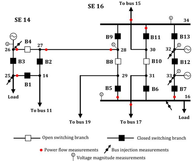
Fig. 2. Details of substations 14 and 16 of IEEE 24-bus test system.
