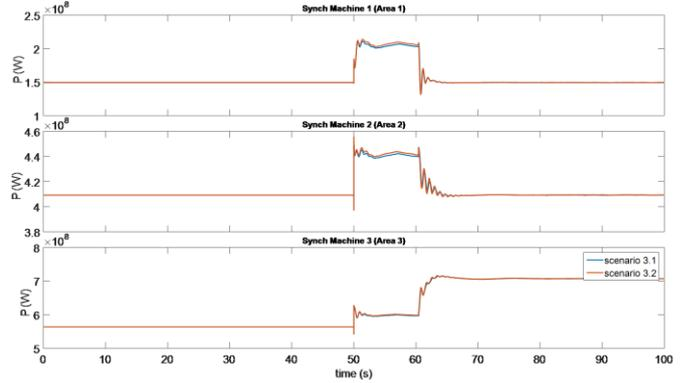
Fig. 14 Synchronous Machine Power (Scenario 3)
