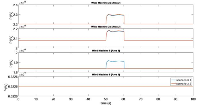
Fig. 15 Wind Machine Power (Scenario 3)
