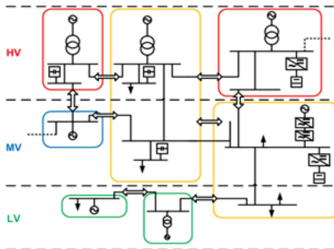
Fig. 1 – Example of a Web-of-Cells power system [3]
