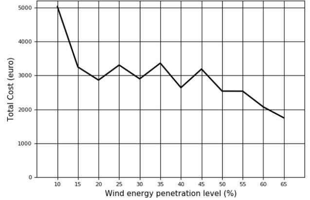
Fig. 6. *s-SCOPF* Cost vs Wind Energy Penetration Level
