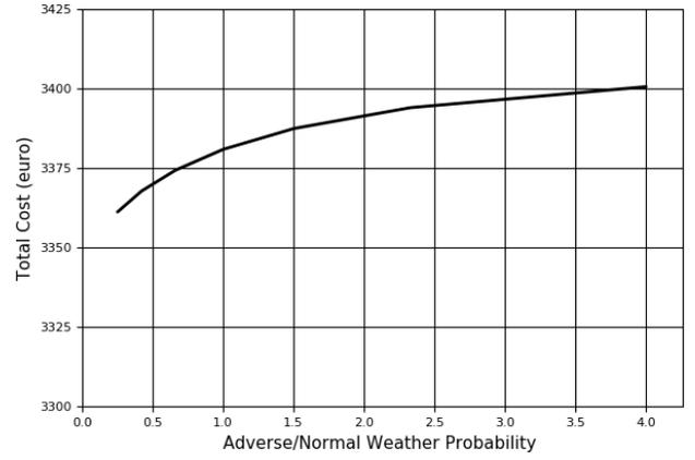
Fig. 5. *s-SCOPF* Cost vs Adverse to Normal Weather Probability Ratio
