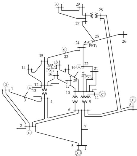
Fig. 8. Modified IEEE 30-bus system; adapted by adding three phase-shifting transformers
