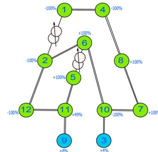
Fig. 9. 12-bus system with two generators (at nodes 9 and 3) and two PST
