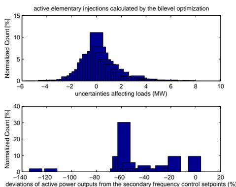
Fig. 5. Elementary injections after the tripping of two generator units
