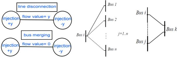
Fig. 3. Compensation injections and fictitious lines to simulate line disconnection/switching and bus merging/splitting
