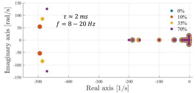
Fig. 3. Evolution of the eigenvalues as the level of VGT increases
