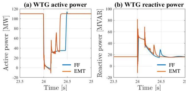
Fig. 6. FF and EMT simulation for scenario 35%. (a) WTG active power, (b) WTG reactive power.
