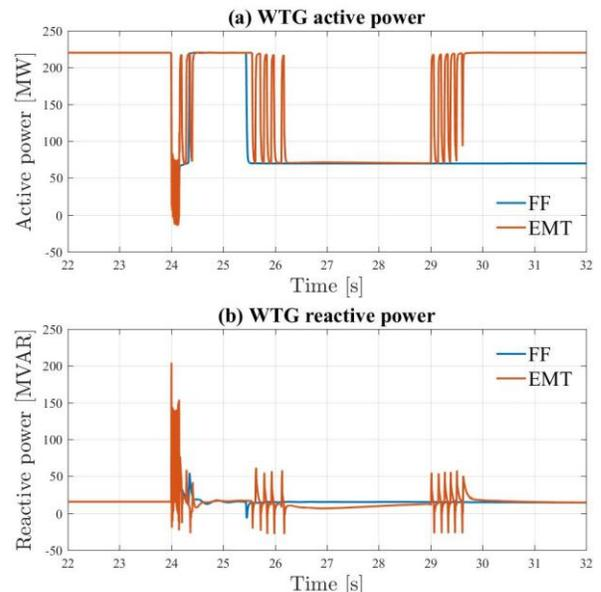
Fig. 8. FF and EMT simulation for scenario 70%. (a) WTG active power (b) WTG reactive power.
