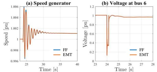
Fig. 4. FF and EMT simulation for base scenario. (a) Speed of generator G2, (b) Voltage at bus 6.
