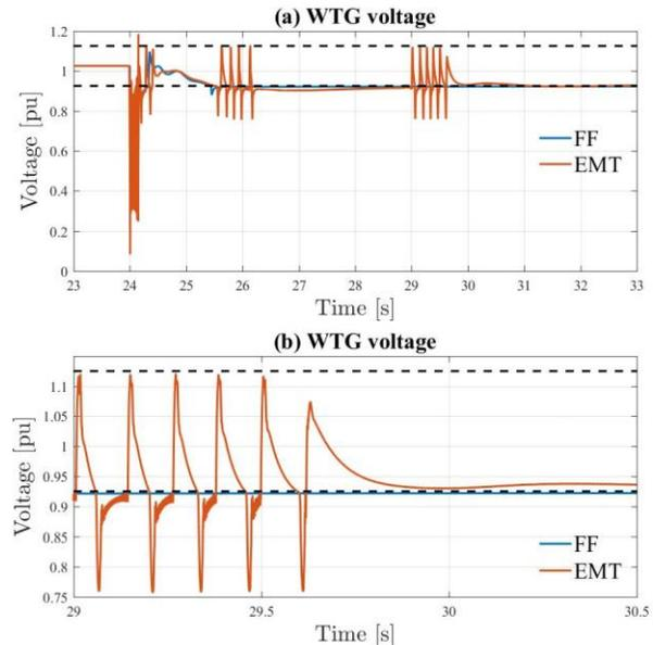
Fig. 7. (a) Voltage at the terminals of the WTG for scenario 70%, (b) Zoom of the voltage.
