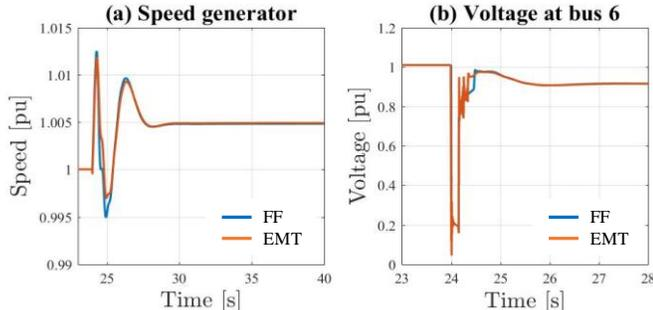
Fig. 5. FF and EMT simulation for scenario 35%. (a) Speed of generator G2, (b) Voltage at bus 6.
