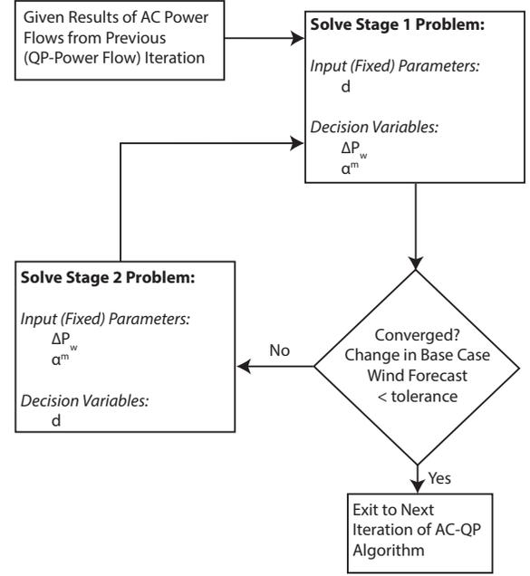
Fig. 2. Iterative solution algorithm for bilinear terms in constraints (4a) and (4b).
