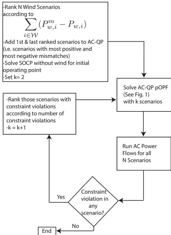
Fig. 3. AC-QP pOPF algorithm for  $N$  scenarios. The QP solved at each iteration focuses on wind power maximization.
