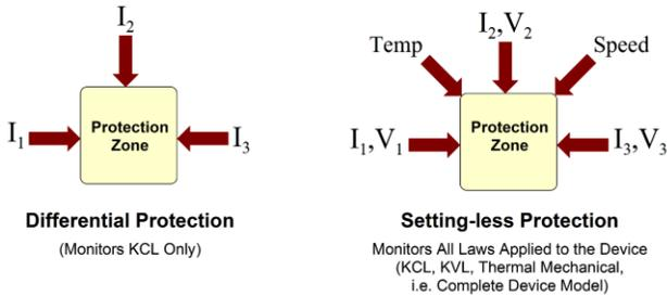
Figure 1: Evolution of the Differential Protection Function [15]
