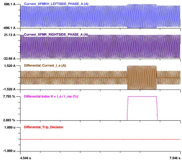
Figure 7: Results of the Differential Protection Scheme
