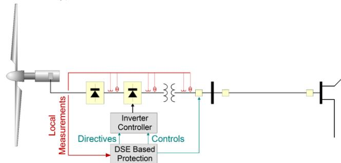
Figure 9: Example of CIG Integrated Protection and Control
