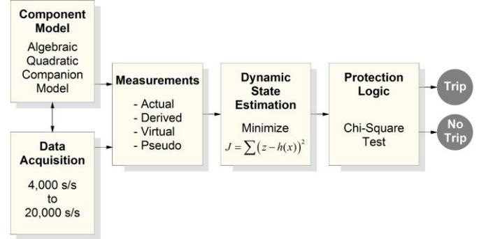
Figure 2: Dynamic State Estimation Based Protection Method
