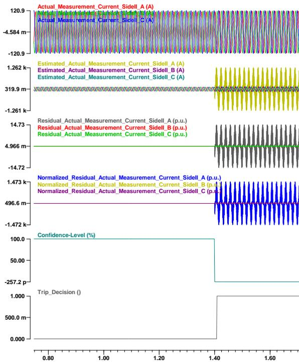
Figure 6. Phase A-N Internal Fault at 1.4s
