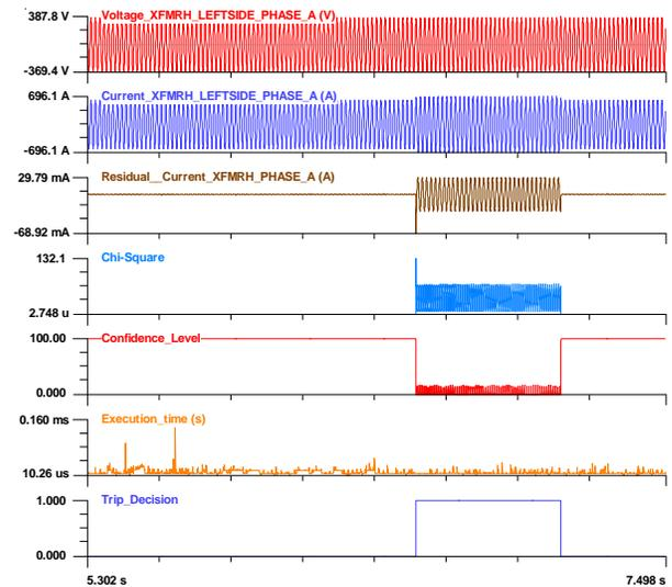
Figure 8: 5% Internal Turn-Ground Fault of Transformer
