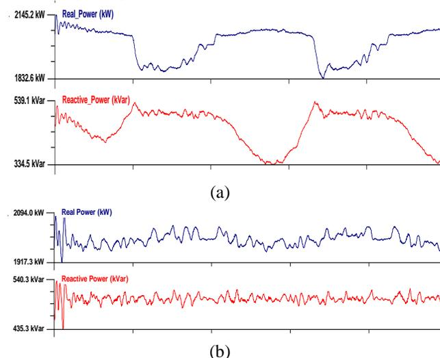
Figure 10: Inverter Real and Reactive Power during a Disturbance Without Integrated Protection & Control (a), with proposed system (b)
